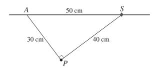
A particle P of weight 5 N is attached to one end of each of two light inextensible strings of lengths 30 cm and 40 cm. The other end of the shorter string is attached to a fixed point A of a rough rod which is fixed horizontally. A small ring S of weight W N is attached to the other end of the longer string and is threaded on to the rod. The system is in equilibrium with the strings taut and AS = 50 cm (see diagram).
